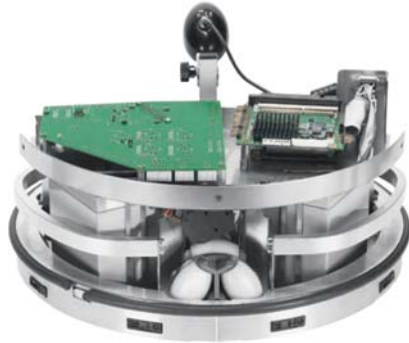
Fig. 5. Controller of Robotino ® consists of an embedded PC and a microcontroller interface board.
